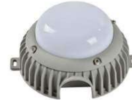
Model No: HO-DL-020-5 Power: 5W Bridgelux/Osram/Epistar 1W/Pcs 5Pcs Size: \phi 140 \times 80 mm Beam Angle: 180° CCT: 2500K/3000K/4000K/Red Blue/ Green
